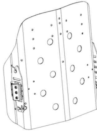
The Prism Hardware offers users a full 5" range of forward and rear adjustability
