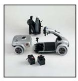
Disassembly Into Five Parts
